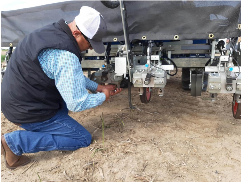
Photo 6. Pacific Ag Rentals technician is showing how to attach the extra camera and robotic arm system for extended length of the machine to cover more rows.
